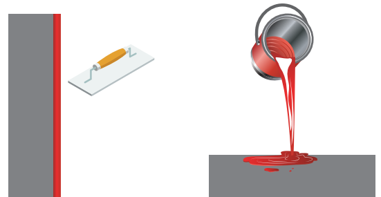
Vertical Wall Trowel Application
